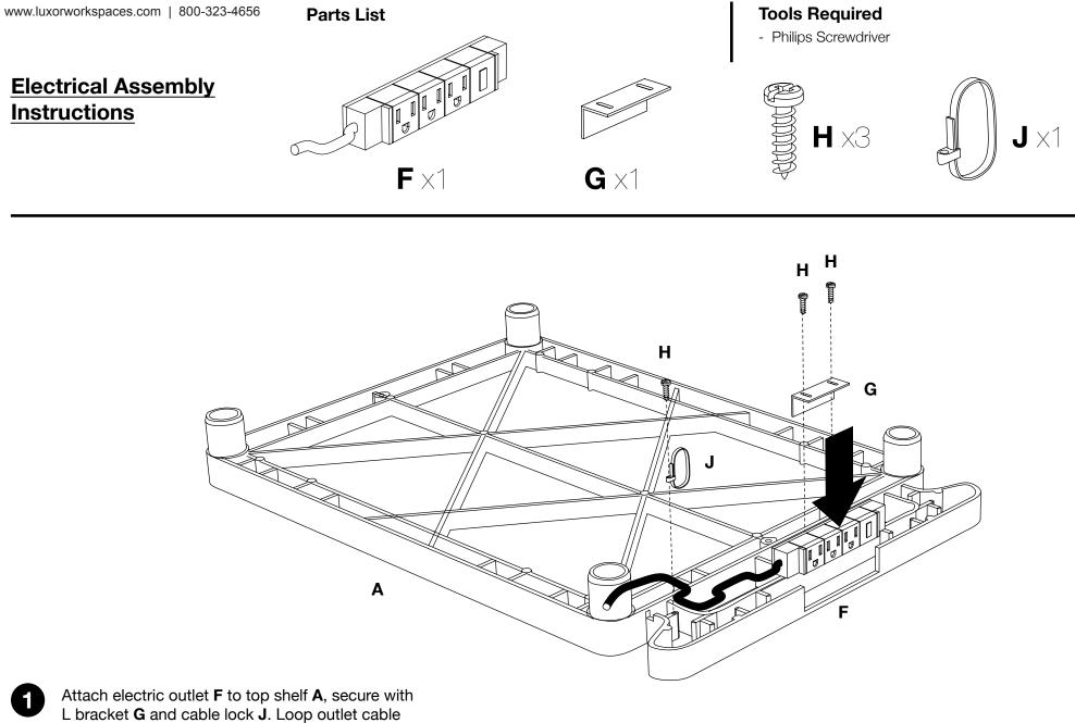
L bracket **G** and cable lock **J**. Loop outlet cable **F** through cable lock **J** and the inserts on shelf **A**. Screw L bracket **G** and cable lock **J** onto top shelf **A** with screw **H** and a philips screwdriver.
